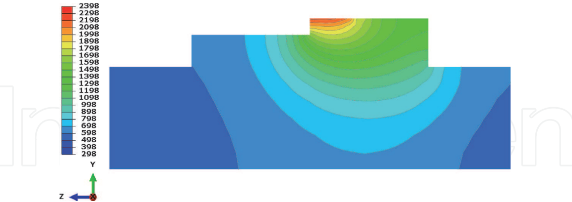
Figure 7. Contour plots of temperature field and isotherms of the substrate and deposits from side view at t = 4.5\text{ s} (Case 1).
