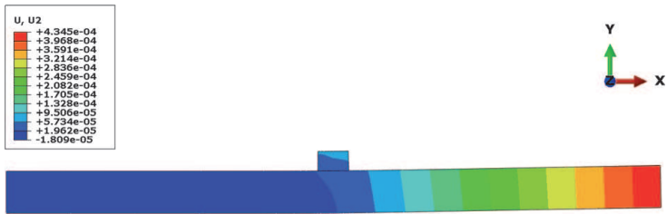
Figure 13. Deflection of substrate along y (m).
