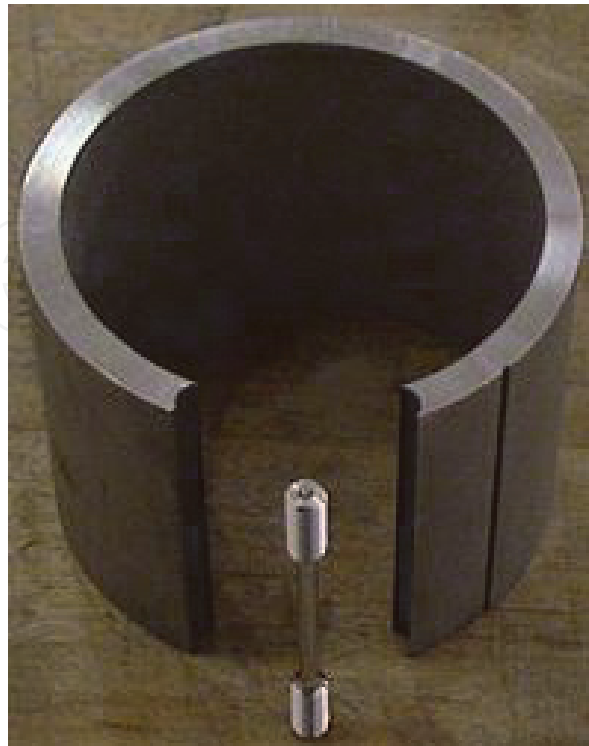
Figure 5. Axial tensile specimen extraction from wall material.
