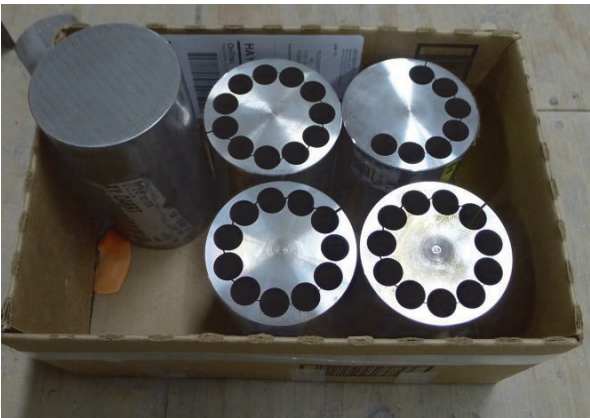
Figure 3. Axial tensile specimen extraction from bar stock.
