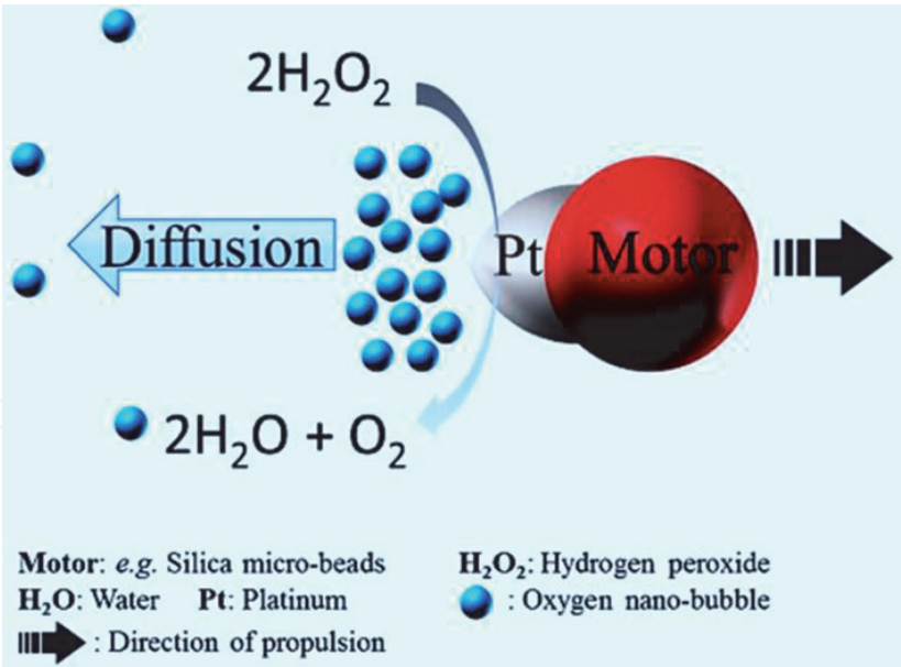
Figure 4. Schematic diagram of a micro/nanomotor propelling under the diffusiophoresis propulsion mechanism. Copyright 2009, Wiley Online Library. Copyright 2011, Frontiers Journals of Higher Education Press.
