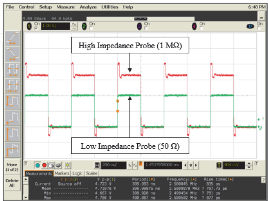
Figure 16. Clock output waveforms comparison at 2.5 MHz.
