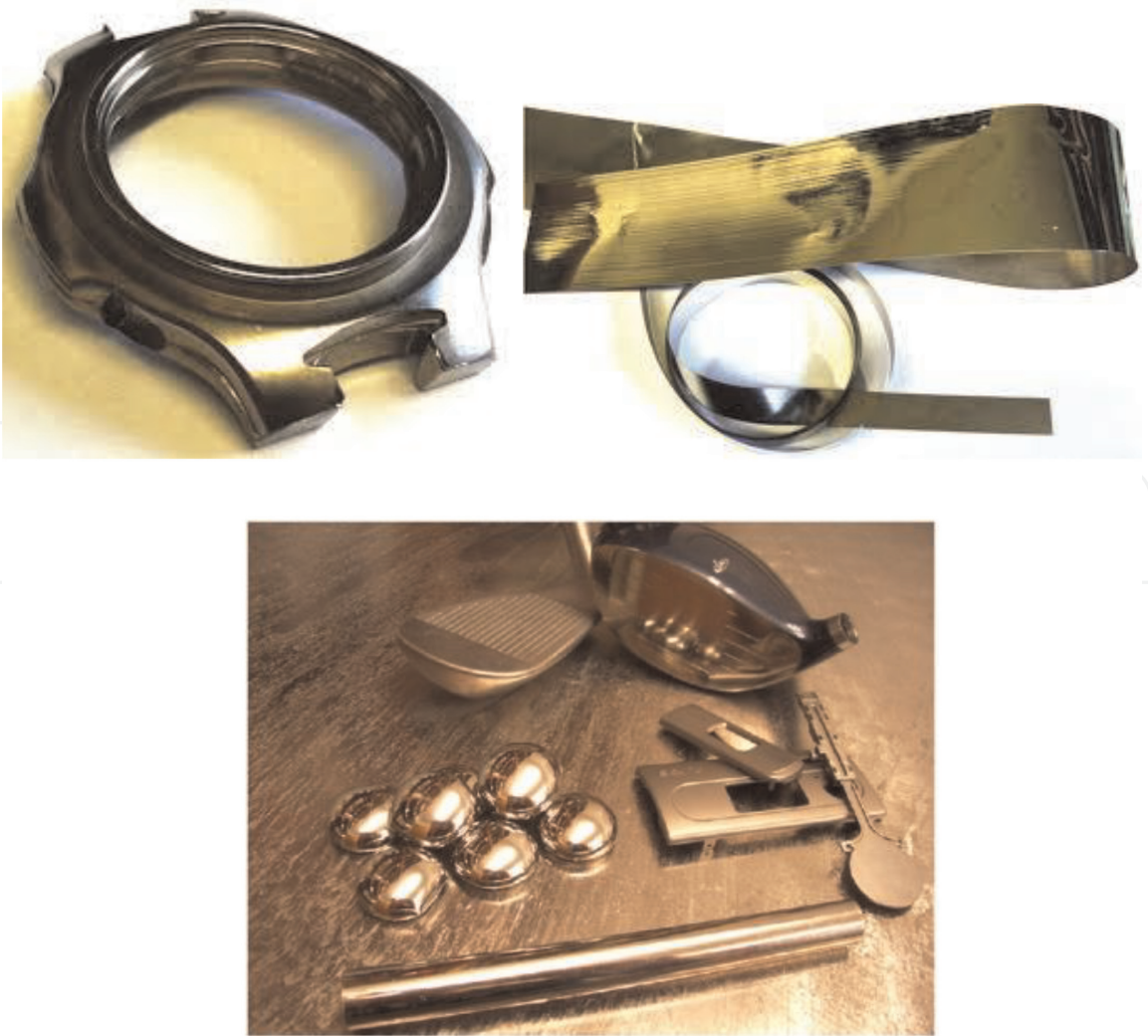
Figure 6. BMG articles fabricated by direct casting method.
