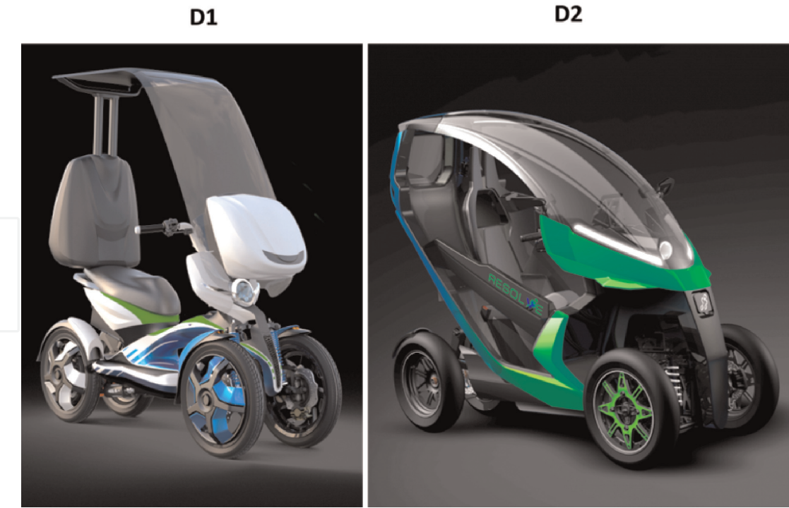
Figure 1. Two demonstrators of narrow tilting vehicle developed in the RESOLVE Project [8].
