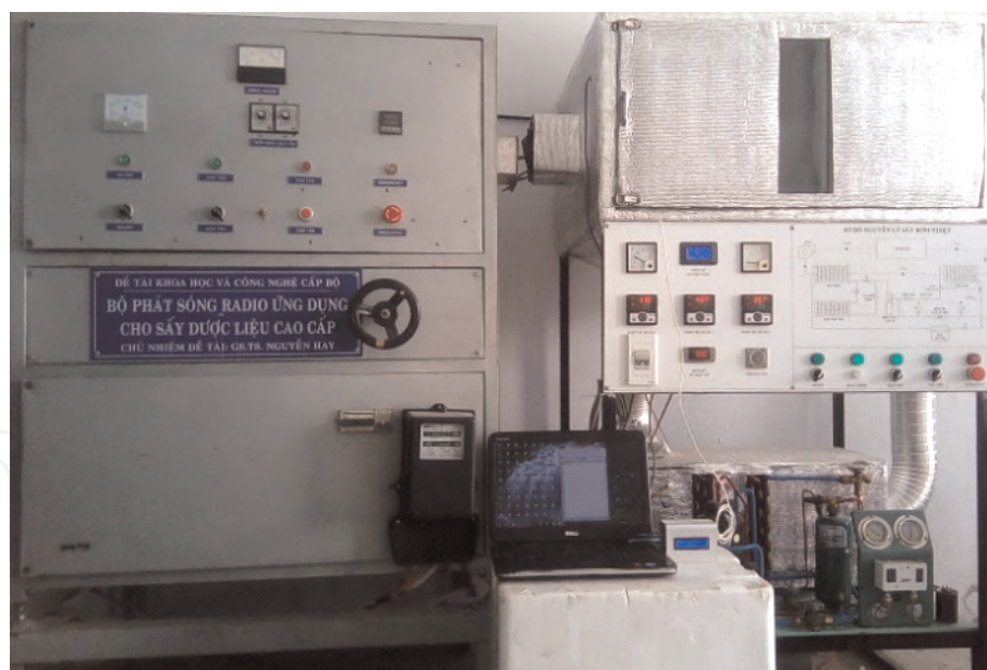
Figure 9. RF-assisted heat pump dryer.
