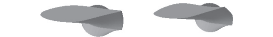
Figure 6. Top view of the blade with S809gx (left) and S809 (right).
