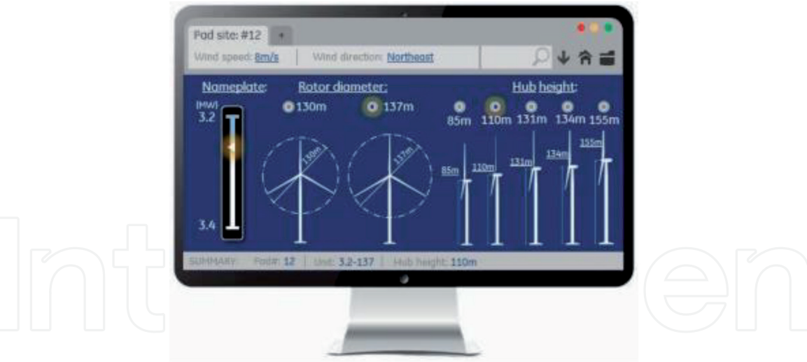
Figure 4. The specifications of wind turbines from the GE 3 MW platform (Credit: GE Renewable Energy).
