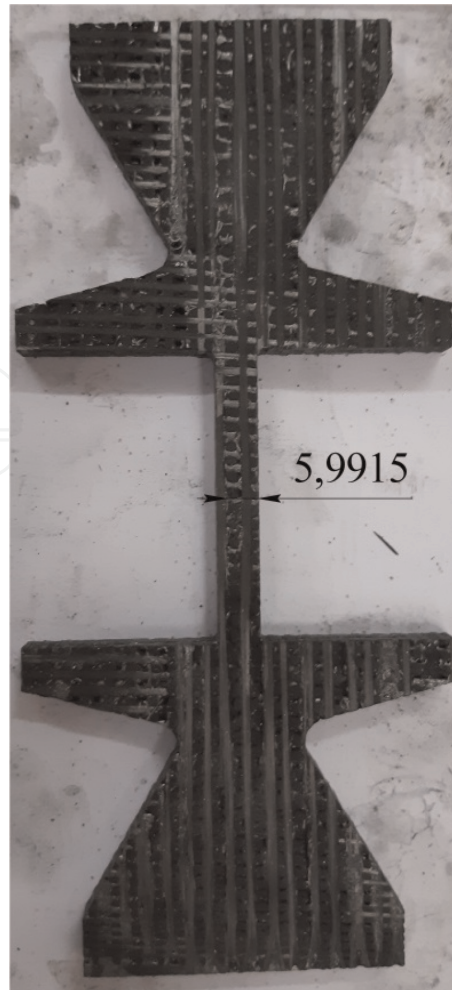
Figure 14. The result of cutting carbon-carbon composites.
