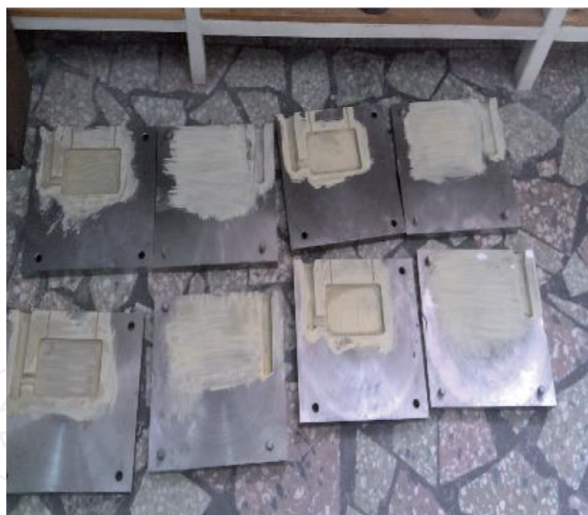
Figure2. Metallic molds for casting Al_{0.8}CrFeCoNi alloy.
