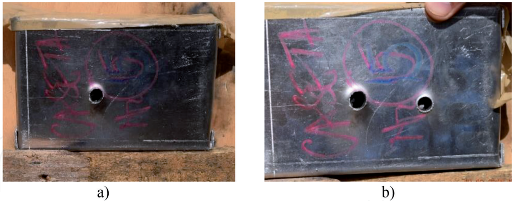
Figure 19. HEA-polymer ballistic package during dynamic tests. (a) after the first firing and (b) after the second firing.
