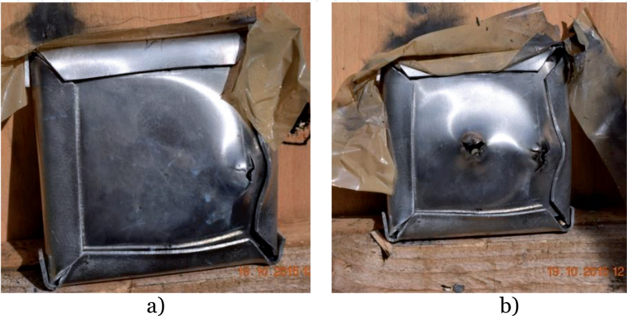
Figure 17. HEA-steel ballistic package during dynamic tests (a) after the first firing and (b) after the second firing.
