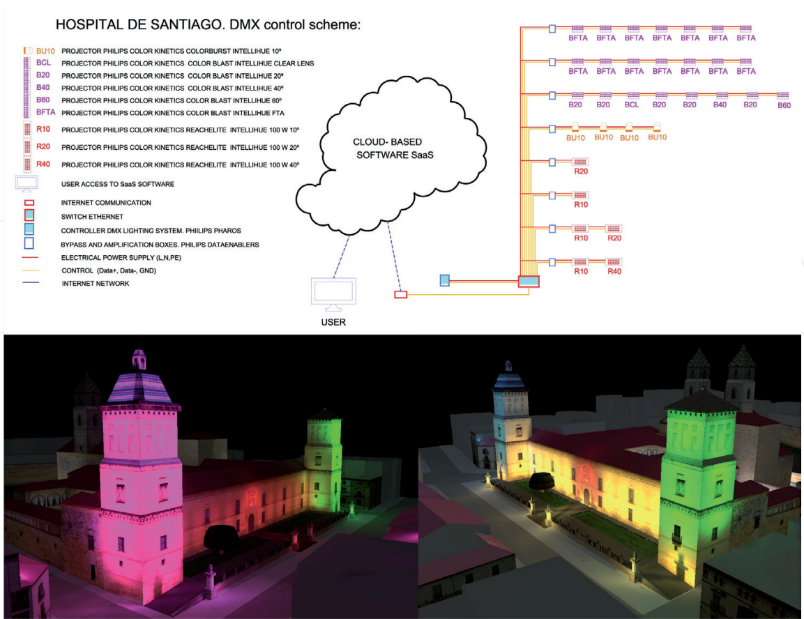
Figure 12. Control scheme. Project of facade illumination Hospital of Santiago Úbeda. Linear installation scheme consisting of Philips Color Kinetics luminaires, 8 DataEnablers, Pharos controller, SaaS, and wiring between power supply (FNP) and data (+, -, G) luminaires. Source: own elaboration.
