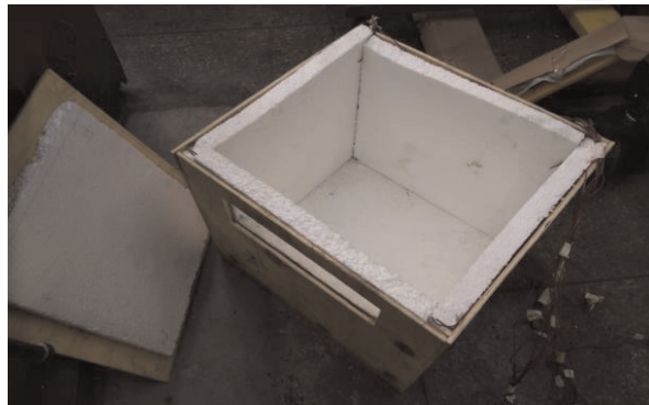
Figure 7. Enclosure for test of thermoelectric air conditioning system.
