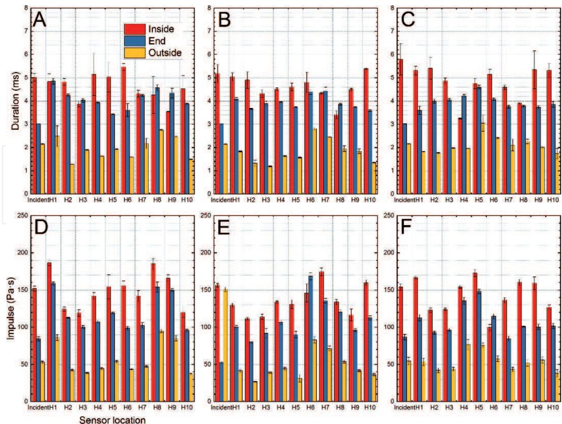
**Figure 5.** The results of the pressure waveforms characteristics quantification. The peak duration and the impulse for the incident and surface mount sensors collected at three different test locations (inside, end and outside) are presented ( $n = 4$ ). The headform orientation in these experiments was  $0^\circ$  (A, C),  $90^\circ$  (B, E), and  $180^\circ$  (D, F).
