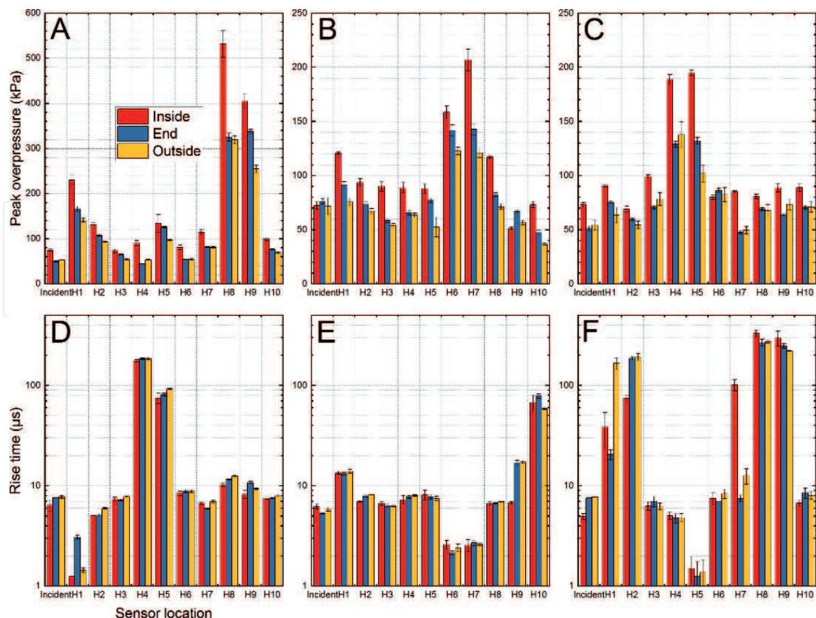
**Figure 4.** The results of the pressure waveforms characteristics quantification. The peak overpressure and the rise time for the incident and surface mount sensors collected at three different test locations (inside, end and outside) are presented (n = 4). The headform orientation in these experiments was 0° (A, C), 90° (B, E), and 180° (C, F).
