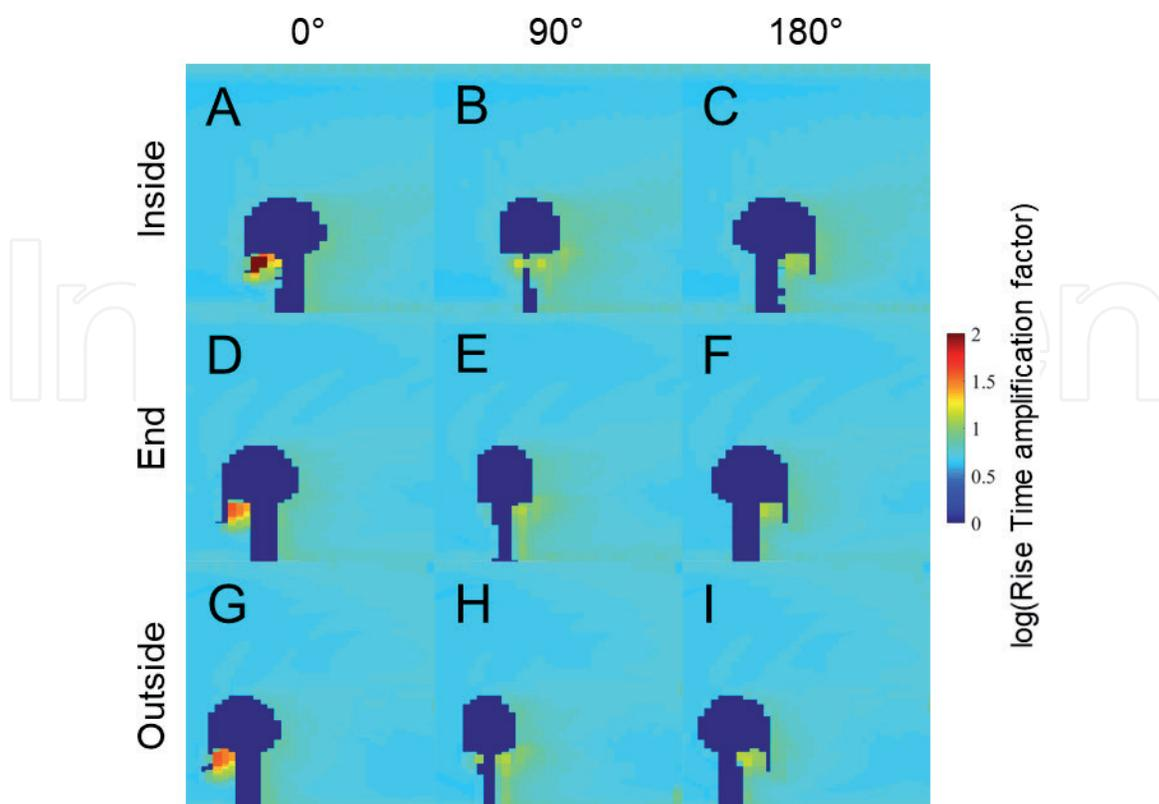
**Figure 10.** Spatial distribution of the rise time amplification factors for the 140 kPa exposures in the region surrounding the headform for three specimen locations and for three headform orientations. Data are reported as the log of the rise time amplification factor, indicated the order of magnitude of the change.
