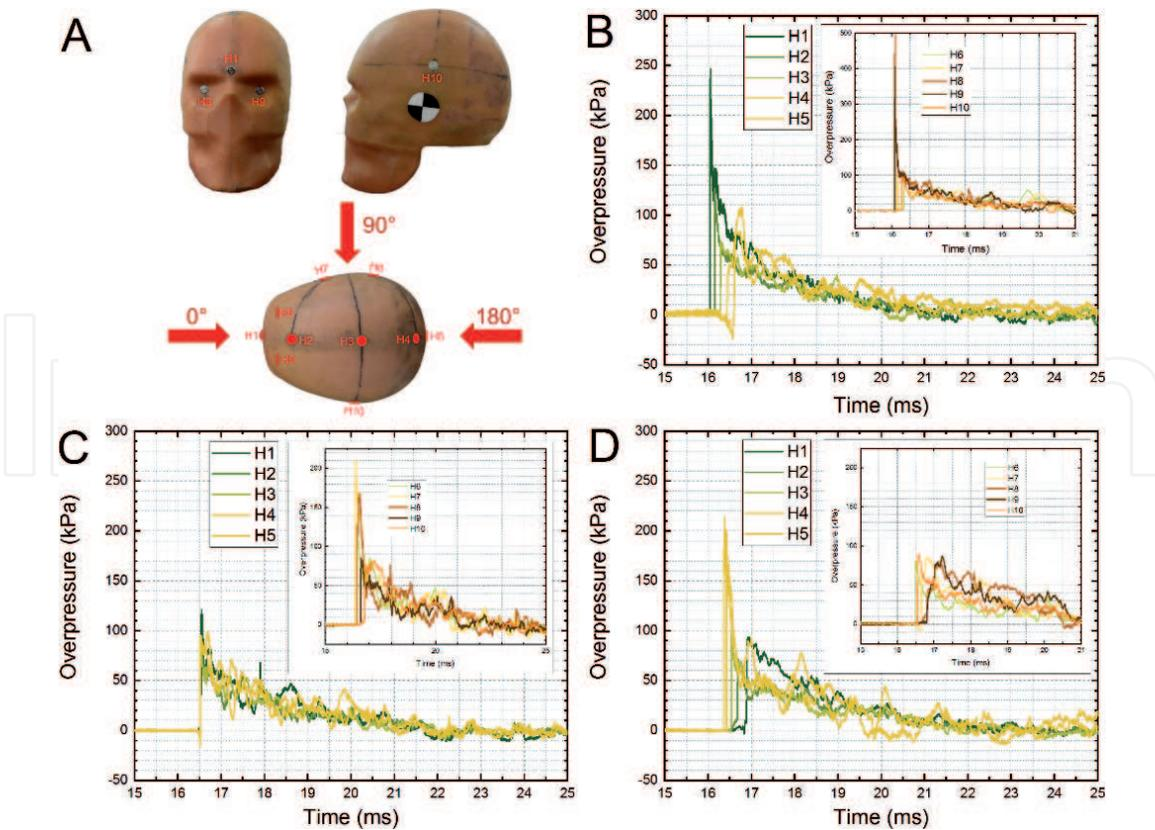
**Figure 2.** The schematic representation of the pressure sensor distribution on the headform (A). The direction of the shock wave propagation in experiments where the headform was rotated in 90° intervals is illustrated. The experimental pressure waveforms collected at 70 kPa nominal shock wave intensity by the surface sensors to three headform orientations: (B) 0°, (C) 90°, and (D) 180° with respect to the direction of the shock wave propagation.
