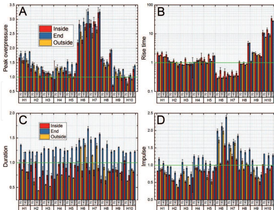
**Figure 6.** The results of the pressure waveform characteristics quantification for headform mounted sensors. The normalized peak overpressure (A), rise time (B), duration (C) and impulse (D) are presented ( $n = 4$ ) for experiments where the headform was mounted at 90° orientation. The normalization allows comparison of the data quantified for three nominal shock wave intensities: 70, 140 and 210 kPa.
