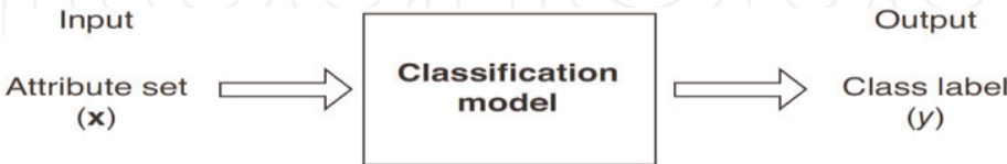
Figure 1. Process of training the objective function f in which each attribute x is mapped.
