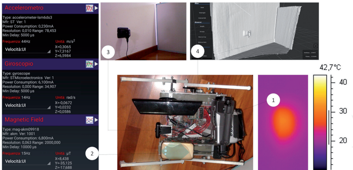
Figure 4. Sensor installation on the inspection robot.
