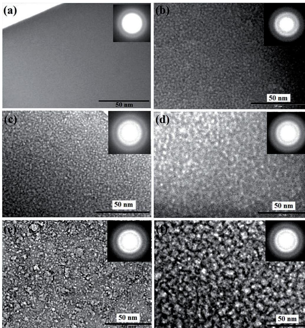
**Figure 3.** Bright-field TEM microstructures and the corresponding selected area diffraction patterns (shown in inset) of  $\text{Ce}_{75}\text{Al}_{25-x}\text{Ga}_x$  alloys with (a)  $x = 0$ , (b)  $x = 0.1$ , (c)  $x = 0.5$ , (d)  $x = 1$ , (e)  $x = 2$ , and (f)  $x = 4$  (reprinted with kind permission from Reference [25], copyright 2016, Elsevier).
