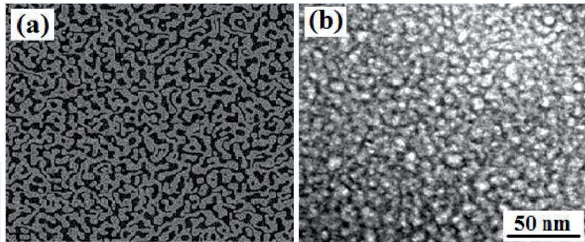
**Figure 8.** Comparison of experimental and theoretical phase field model of phase separation in spinodal decomposition (a) numerical simulated microstructure with 43% and 57% phase fraction and (b) experimental microstructure of  $Ce_{75}Al_{21}Ga_4$  alloy.
