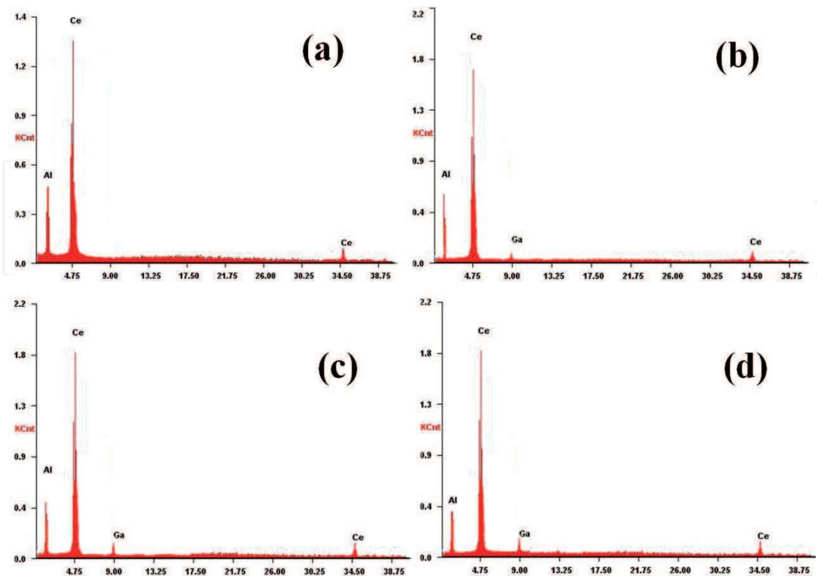
**Figure 4.** Energy dispersive spectra of the melt-spun  $Ce_{75}Al_{25-x}Ga_x$  alloys for (a)  $x = 0$ , (b)  $x = 0.5$ , (c)  $x = 1$ , and (d)  $x = 4$  alloys (reprinted with kind permission from Reference [25], copyright 2016, Elsevier).
