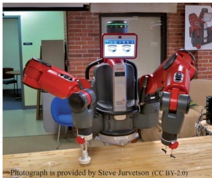
Figure 7. A collaborative robot: Baxter robot [52].
