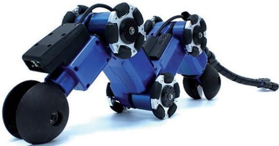
Figure 7. A multi-link-articulated wheeled-type in-pipe robot named AIRo-2.2 [20].
