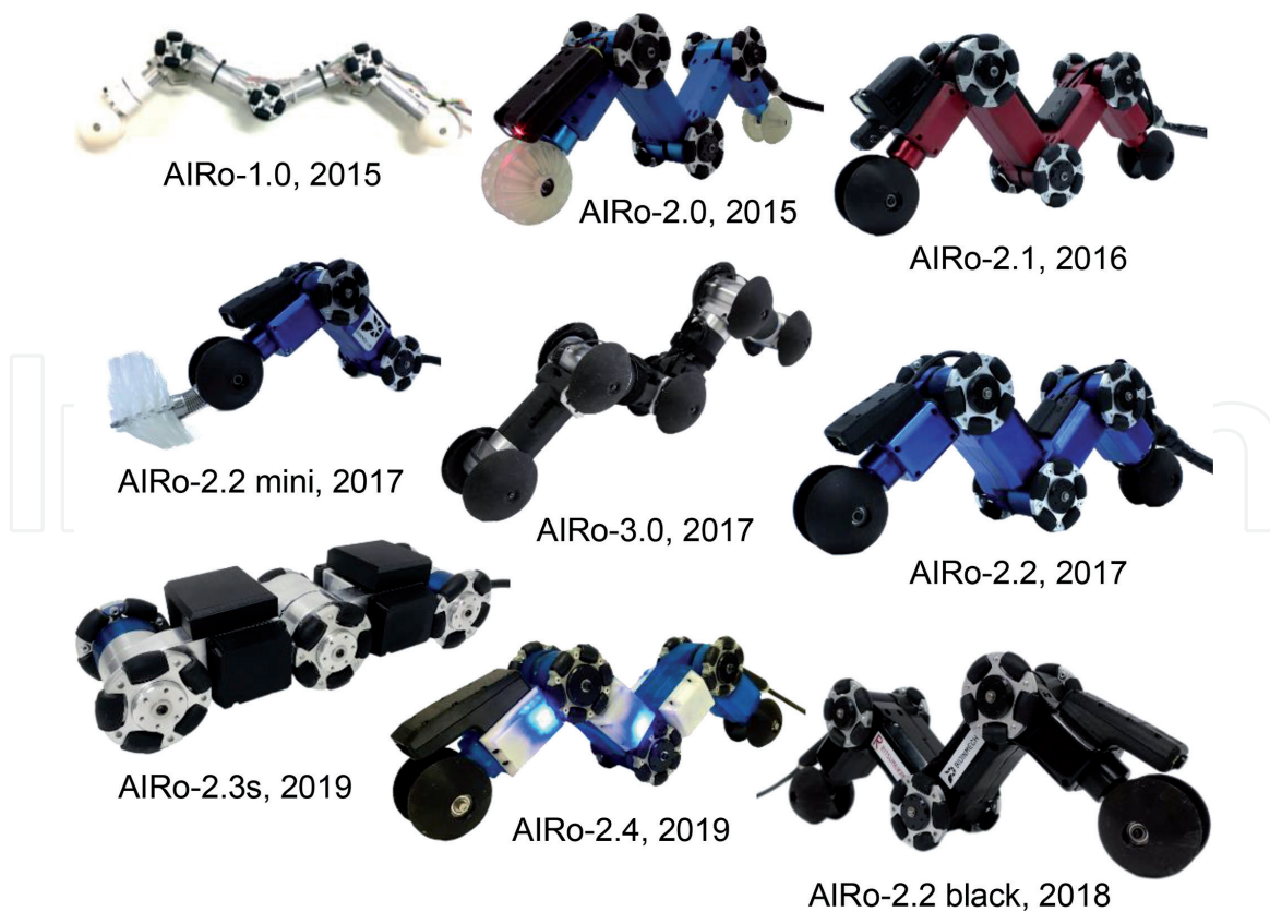
Figure 11. Multi-link-articulated wheeled-type in-pipe robots in the AIRo-series developed by the authors.
