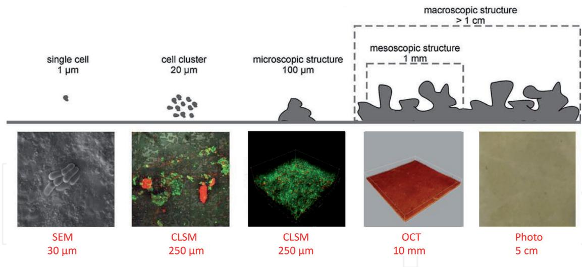
**Figure 4.** Techniques to characterize fouling structure at different scales: SEM, scanning electron microscopy; CLSM, confocal laser scanning microscopy; and OCT, optical coherence tomography. Adapted from Wagner et al. [18].
