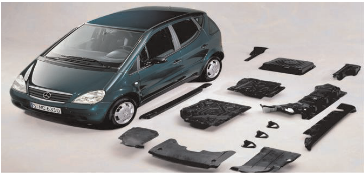
Figure 2. Mercedes-Benz A-Class vehicle components made of flax fiber composites [46].
