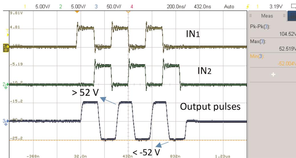
**Figure 18.** Measured input signals and output waveform of the proposed pulse generator under a 1-K ohm resistance in parallel with a 220-pF capacitance load.
