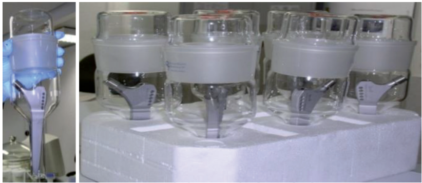
Figure 17. Glass reactors for cation extraction tests.
