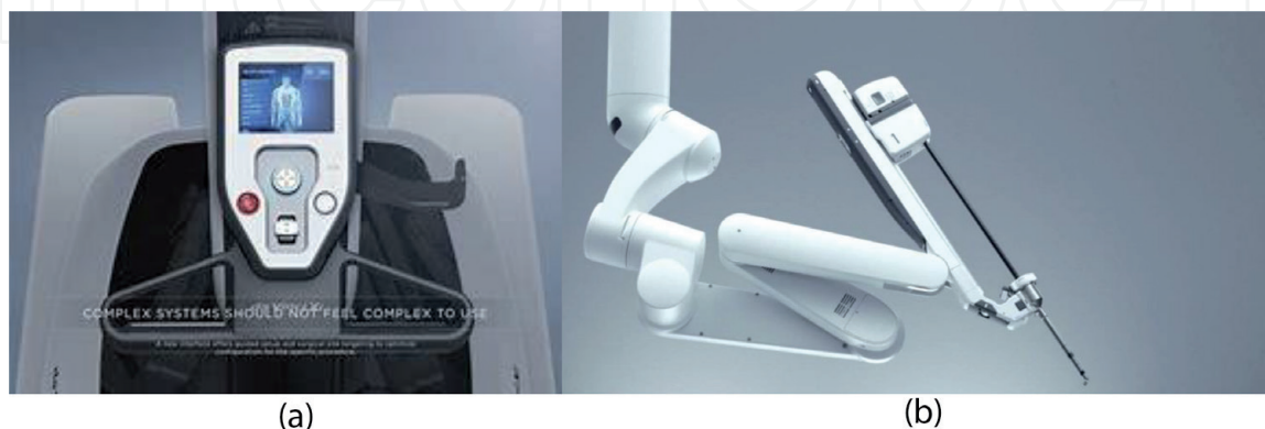
Figure 5. The patient cart. (a) The visual pad on the patient cart that allows operator to set the type of surgery to be performed and the handles that allows the patient cart to be moved around theatre. (b) A robotic arm with an instrument in place. The port and instrument clutches can be utilised to move the instrument into the correct position. Setting set-up it must be ensured that the robotic arms are in the correct alignment to avoid unnecessary collisions and clashes between arms.
