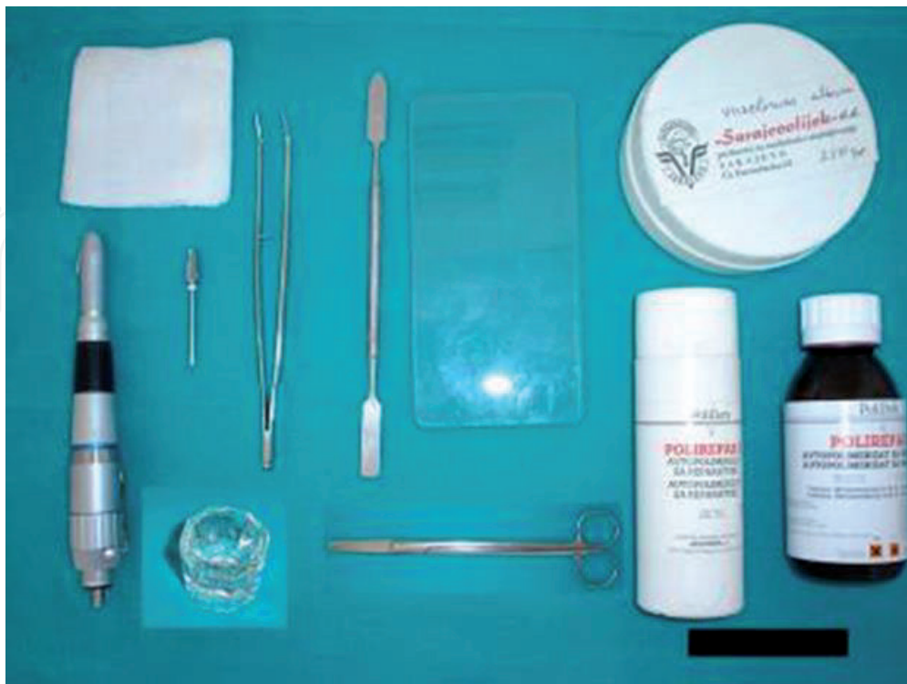
Figure 4. Equipment for creating an acrylic Pfeiffer splint.
