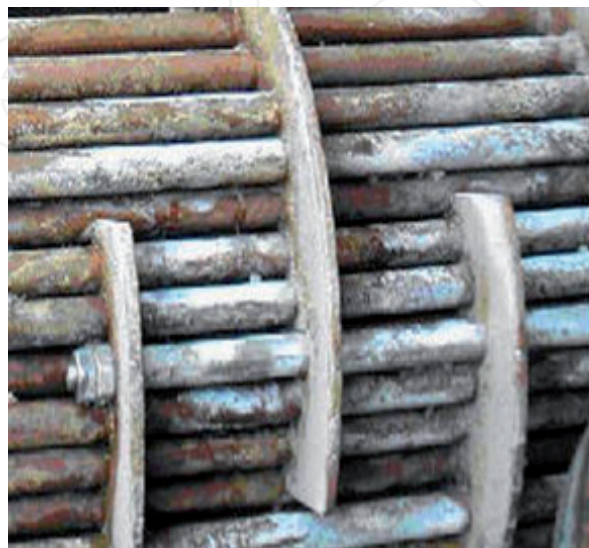
Figure 6. Precipitated salts in the tubes of a heat exchanger (Source: By courtesy of H&C Heat Transfer Solutions Inc).
