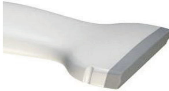
Figure 3. Linear-array probe used for breast shearwave elastography.
