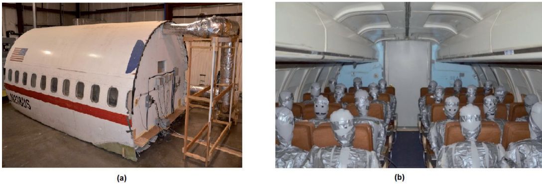
Figure 4. 5-rows B737 (a) exterior and (b) interior with inflatable heated manikins [7].
