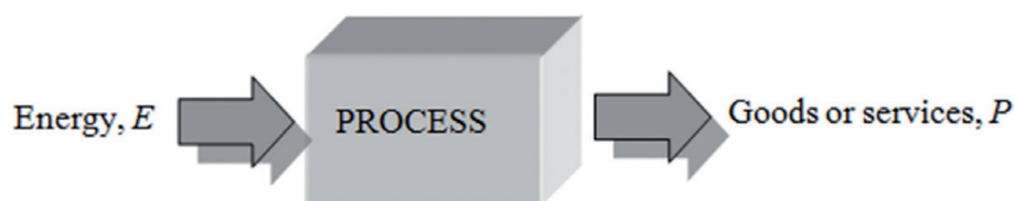
Figure 1. Energy efficiency as the ratio of goods-services provided and the energy input.
