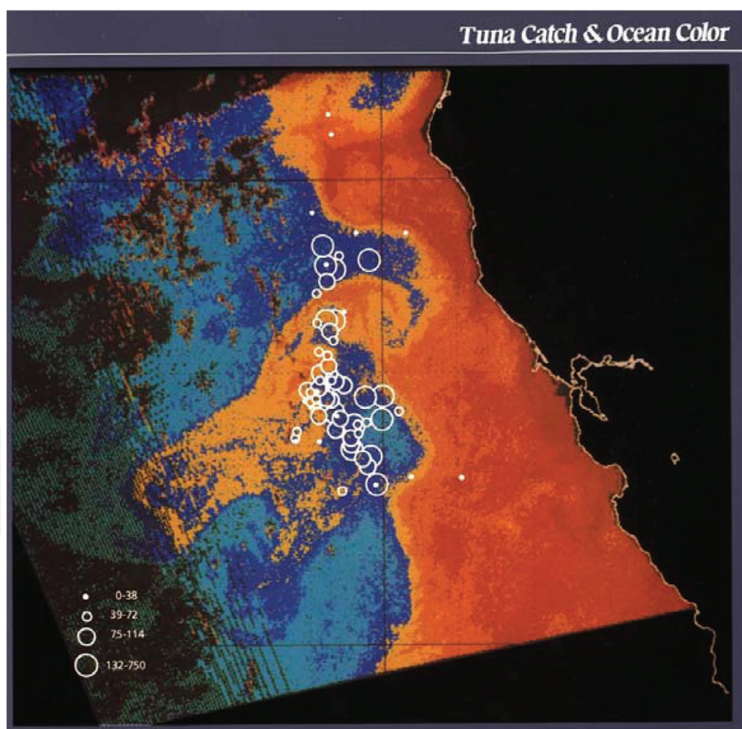
Figure 11. Nimbus-7 coastal zone color scanner (CZCS) satellite image showed locations of fish catch and their relation to the water color and showed a transition from coastal waters (orange color refers to the coastal water with high productivity, and blue color refers to the offshore areas). Source: NASA.
