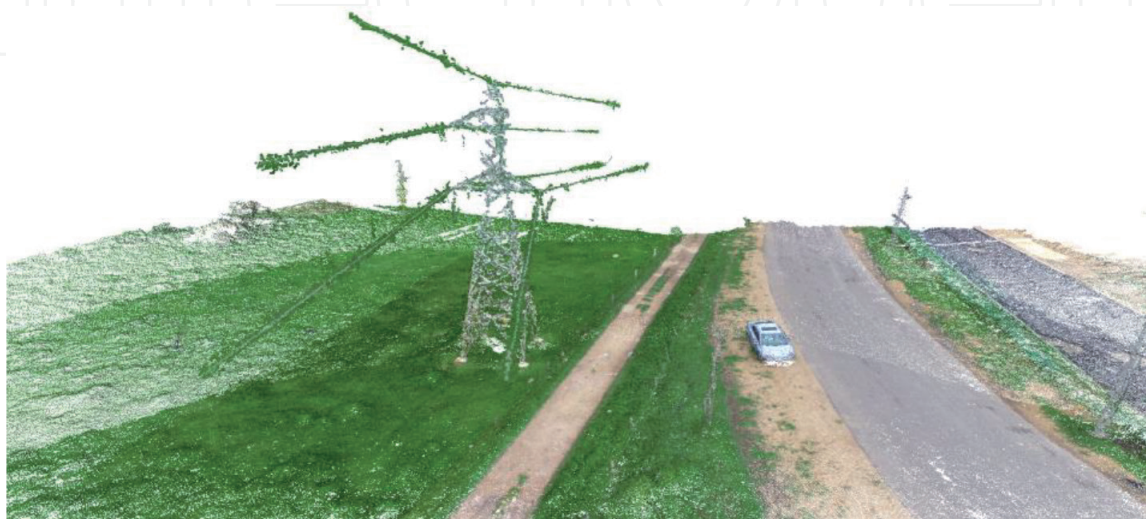
Figure 15. Results of 3D reconstruction of electrical infrastructure.
