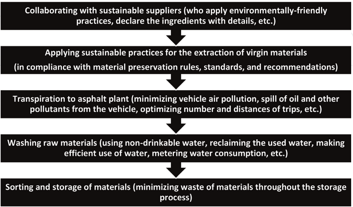
Figure 4. Sustainable procurement process of materials in an asphalt plant.
