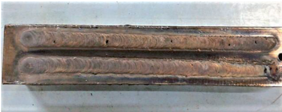
Figure 4. Cu-Sn alloy surface modified with Ni.
