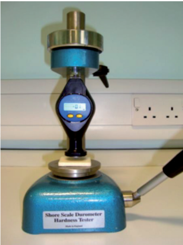
Figure 6. Hardness tester testing hardness of the printed samples.
