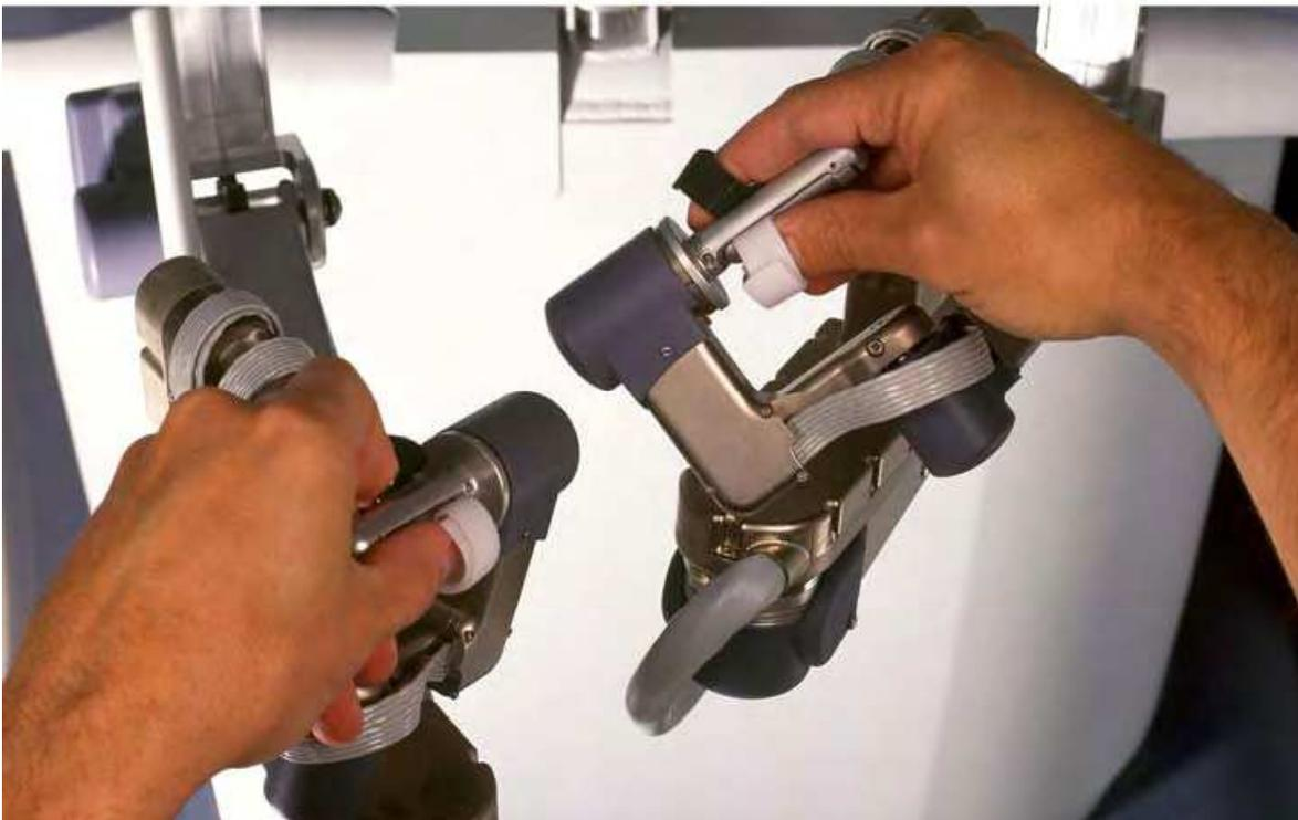
Figure 3. Surgeon's console including operative field view (above) and master controls (below). ©[2007] Intuitive Surgical, Inc
