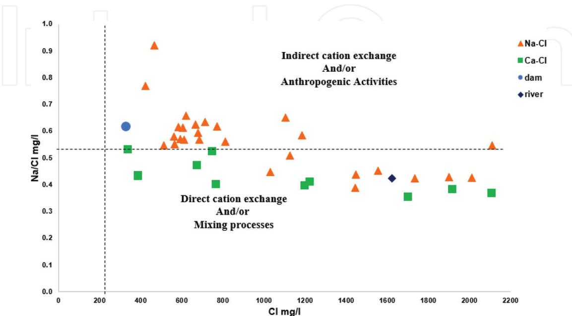
**Figure 5.** Diagram plot of Na/Cl (mg/l) ratio and Cl (mg/l) concentrations for groundwater and surface water samples.
