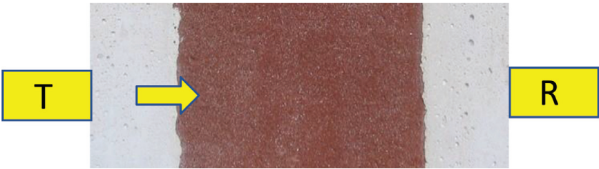
Figure 8. Experimental set-up for ultrasonic characterization tests.
