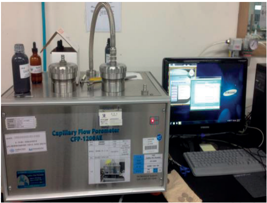
Figure 7. Image of capillary flow porometer, CFP-1200AE.
