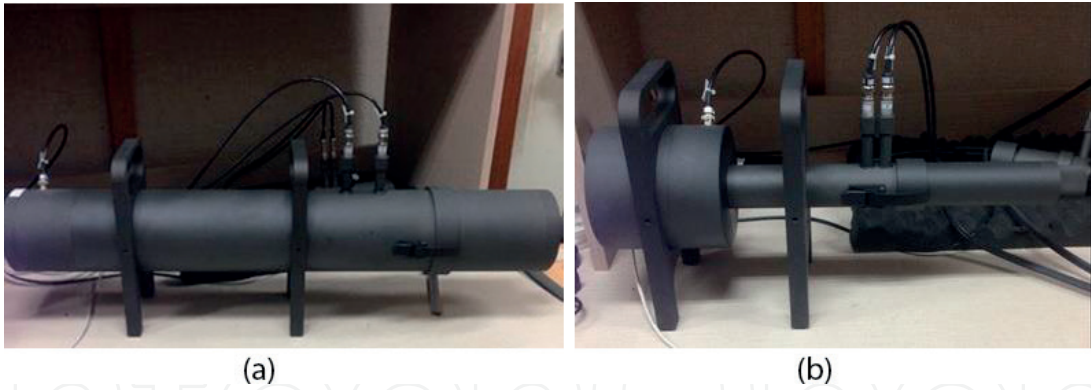
Figure 9. Acoustic duct, SCIEN-9301. (a) Low Frequency and (b) High Frequency.
