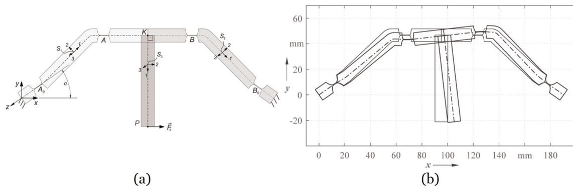
**Figure 12.** Analytical modeling of the Roberts mechanism ( $\beta_1 = 1$ ,  $\beta_h = 0.03$ ): (a) branched mechanism with point  $P$  split up in three individual rods connected at point  $K$ , (b) resulting from MATLAB plot of initial and deflected state for  $u_{xP} = 10$  mm ( $n_{A_0} = 3$ ,  $n_A = 12$ ,  $n_B = 10$ ,  $n_{B_0} = 3$ ).
