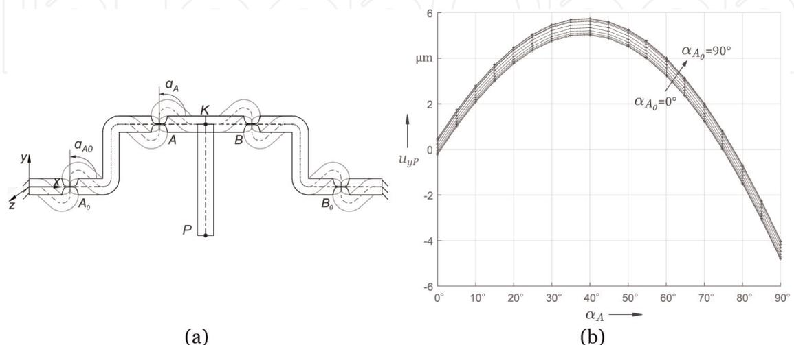
**Figure 13.** Analytical results for the influence of the flexure hinge orientation on the straight-line deviation of a mechanism with power function contours ( $\beta_1 = 1$ ,  $\beta_h = 0.03$ ,  $u_{xP} = 10$  mm): (a) model with two variable orientation angles from  $0^\circ$  to  $90^\circ$  and (b) deviation of  $P$ .
