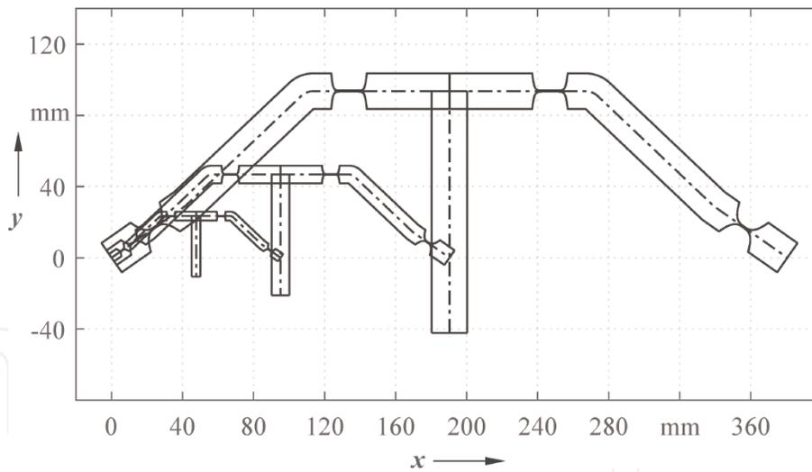
**Figure 14.** Geometric scaling of the compliant Roberts mechanism shown for the factors  $g = 0.5$ ,  $g = 1$ , and  $g = 2$  (mechanism with different power function hinges,  $\beta_1 = 1$ ,  $\beta_h = 0.03$ ).
