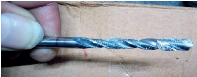
Figure 9. Adhesion of material to the drill bit.
