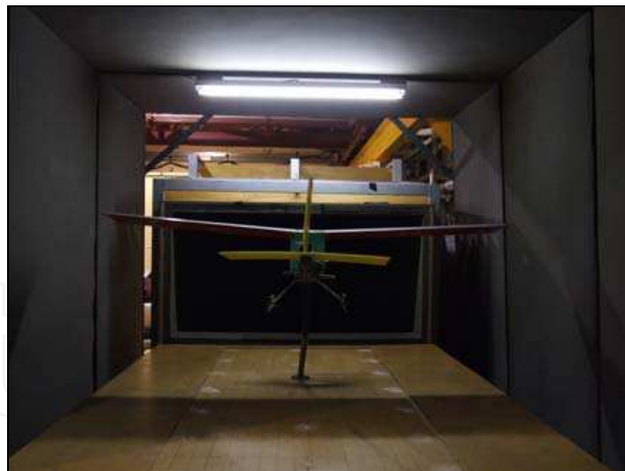
Fig. 14. Wind tunnel test setup
