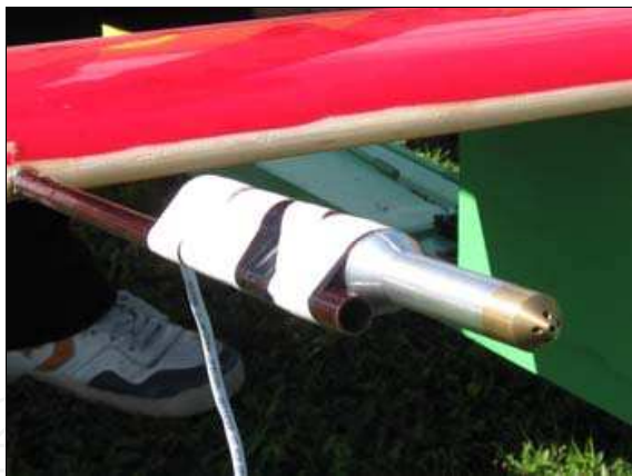
Fig. 6. Wind speed sensor mounting
