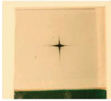
Figure 6. Matched Fourier-plane filter, exposed and developed in the optical path [7].
