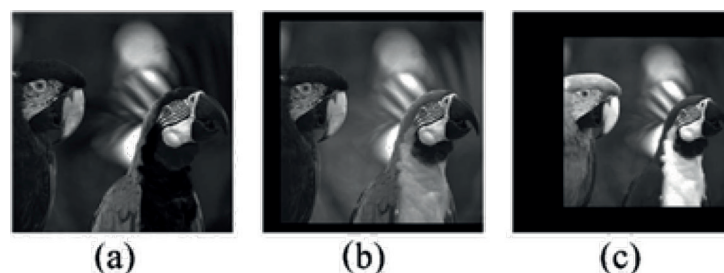
Figure 23. Resizing and repositioning of the input color components allows quick compensation of the chromaticity of holographic projection: (a) blue component; (b) green component; (c) red component [33].
