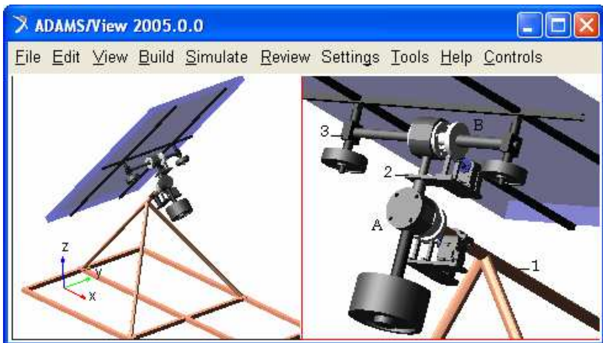
Fig. 5. The MBS mechanical model of the dual-axis tracking mechanism
