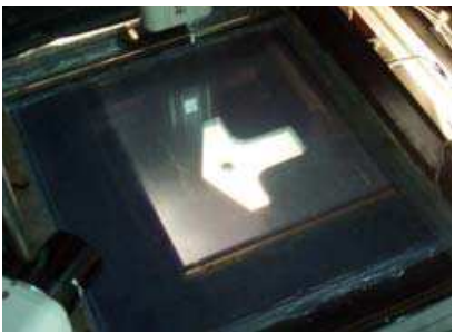
Fig. 3. The LCD photomask of the proposed system
