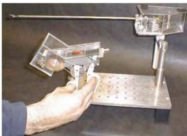
Figure 4. Force controlled gripper designed at the University of Washington (Rosen et al., 1999a)
