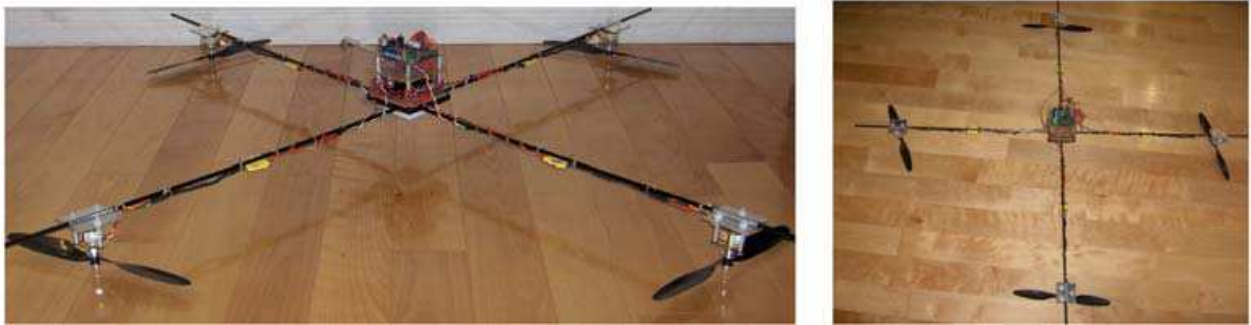
Fig. 15. The quadrotor test-bed.
