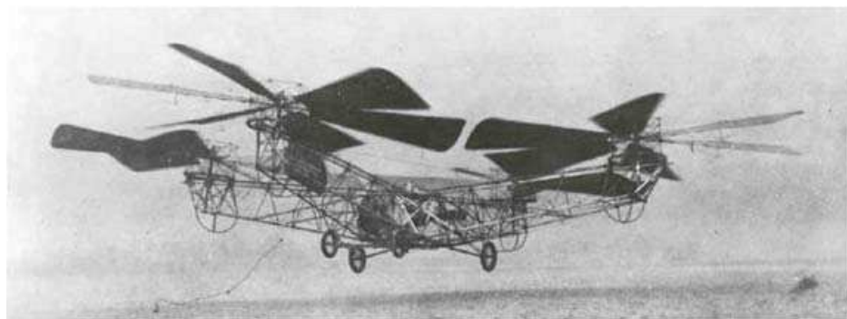
Fig. 2. Quadrotor designed by George De Bothezat, February 21, 1923 Rumerman (2002).
