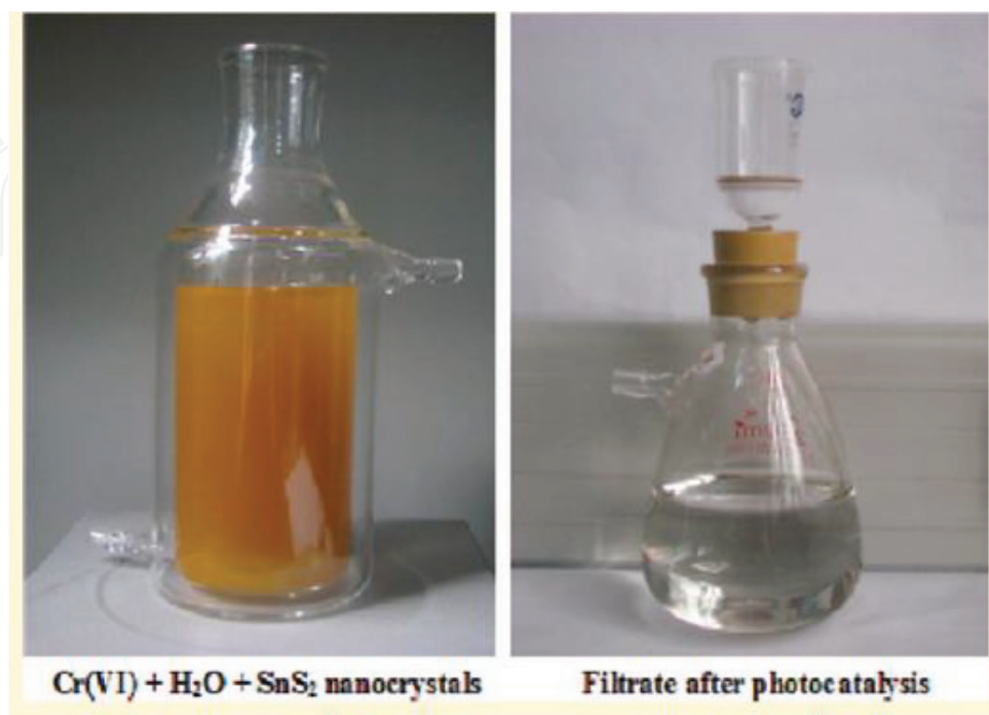
Figure 20. Photodegradation of Cr(VI) in the presence of \text{SnS}_2 . Reproduced with permission from [23].
