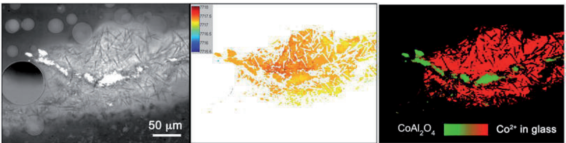
Figure 10. FF-XANES investigation performed on ID21 beamline at ESRF [18]. (a) Transmission image recorded at 7670 eV, (b) edge energy map, (c) phase map obtained from the least squares linear combination fitting (standards \text{CoAl}_2\text{O}_4 and Co in glaze) of each single pixel.
