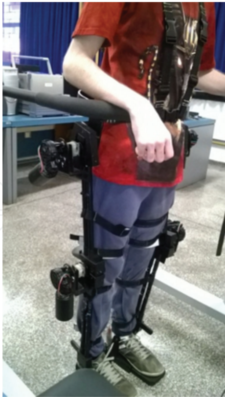
Figure 5. Mechanical structure of the active orthosis with a volunteer on the partial weight support system.
