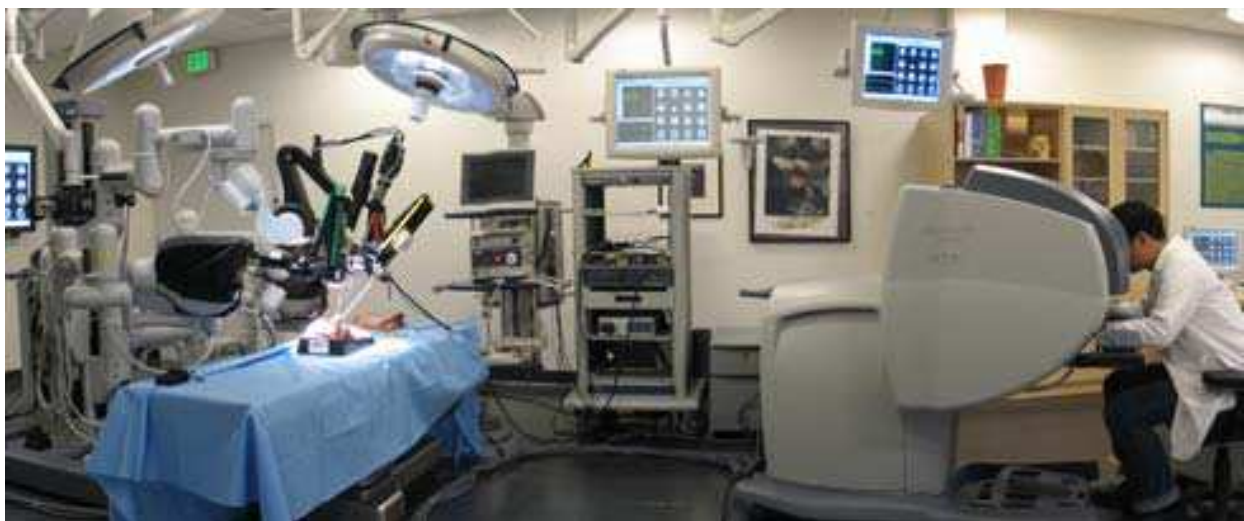
Fig. 4. The da Vinci surgical master (right) and slave (left) platform at the CASIT Center for Advanced Surgical and Interventional Technology at the University of California, Los Angeles.
